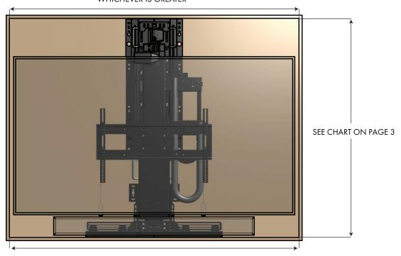
MIN. CEILING COVER CUTOUT WIDTH = W + 2 in [5.1 cm] OR SW + 2 in [5.1 cm] OR 35 in [88.9 cm] WHICHEVER IS GREATER
